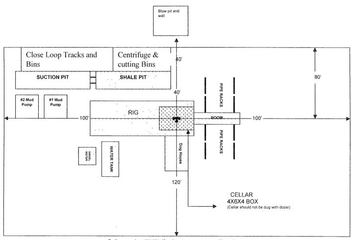
Cellar can be 4X4X4 if using a screw-on wellhead
