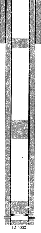
7-7/8" hole @ 4000' 5-1/2" csg @ 4000' w/ 660sx-TOC-Surf-Circ
