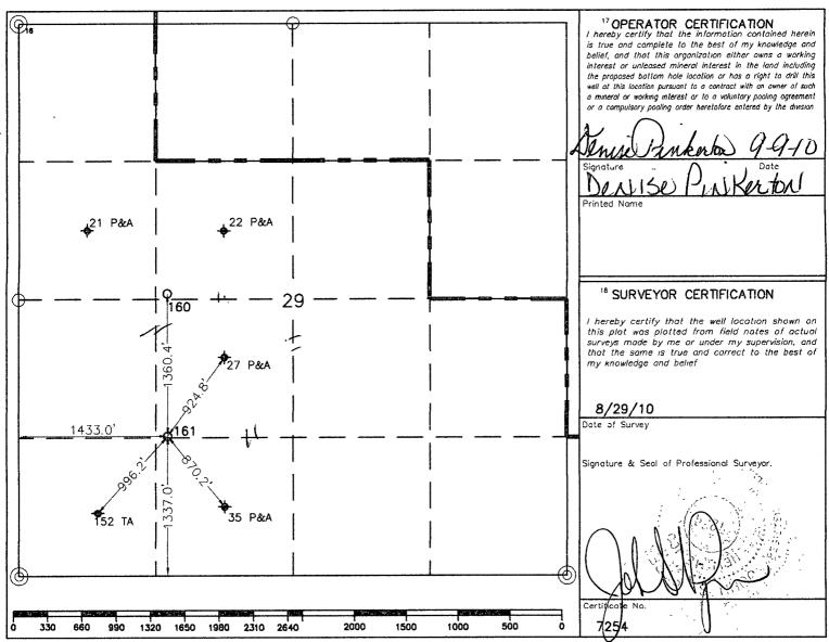
O = Staked Location • = Producing Well • = Injection Well • = Water Supply Well • = Plugged & Abandon Well (iii) = Found Section Corner, 2 or 3" Iron Pipe & GLO B.C. O = Found /4 Section Corner, 1" Iron Pipe & GLO B.C.
