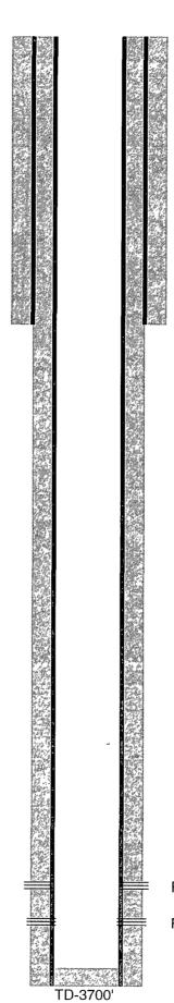
12-1/4" hole @ 1123' 8-5/8" csg @ 1123' w/ 675sx-TOC-Surf-Csg
