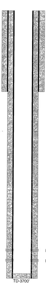
12-1/4" hole @ 1122' 8-5/8" csg @ 1122' w/ 675sx-TOC-Surf-Csg
