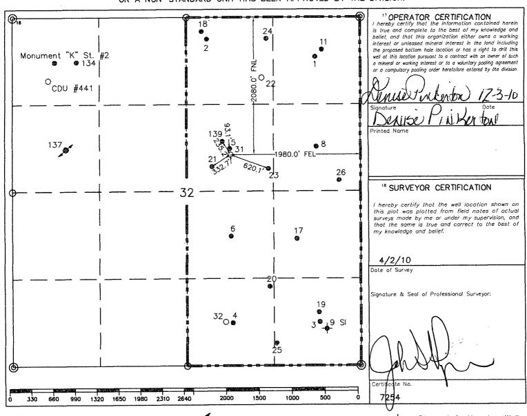
O = Staked Location • = Producing Well = Injection Well • = Water Supply Well • = Plugged & Abandon Well O = Found /4 Section Corner, 1" Iron Pipe & GLO B.C. (O) = Found Section Corner, 2 or 3" Iron Pipe & GLO B.C.
