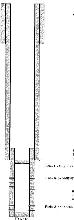
17-1/2" hole @ 1275' 13-3/8" csg @ 1275' w/ 850sx-TOC-Surf-Circ
