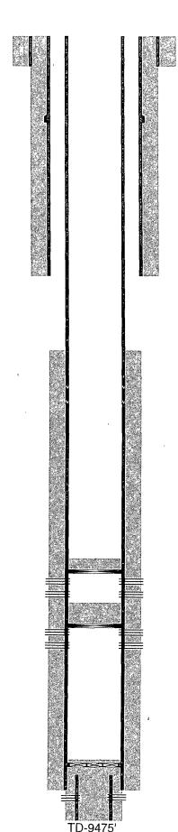
17-1/2" hole @ 305' 13-3/8" csg @ 305' w/ 300sx-TOC-Surf-Circ
