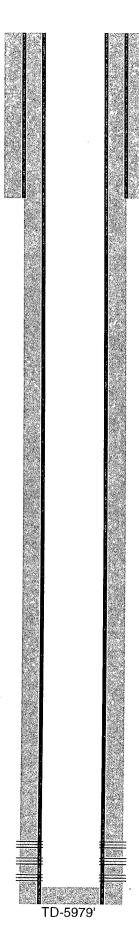
11" hole @ 1092' 8-5/8" csg @ 1092' w/ 635sx-TOC-Surf-Circ
