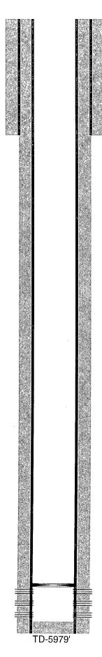
11" hole @ 1092' 8-5/8" csg @ 1092' w/ 635sx-TOC-Surf-Circ
