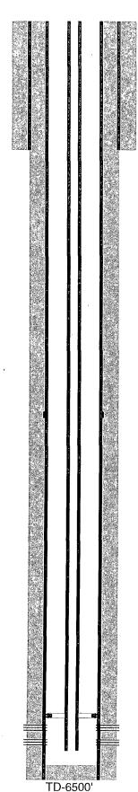
11" hole @ 1100' 8-5/8" csg @ 1100' w/ 500sx-TOC-Surf-Circ
