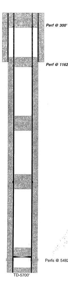
12-1/4" hole @ 1112' 8-5/8" csg @ 1112' w/ 650sx-TOC-Surf-Circ
