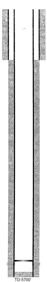
12-1/4" hole @ 1112' 8-5/8" csg @ 1112' w/ 650sx-TOC-Surf-Circ
