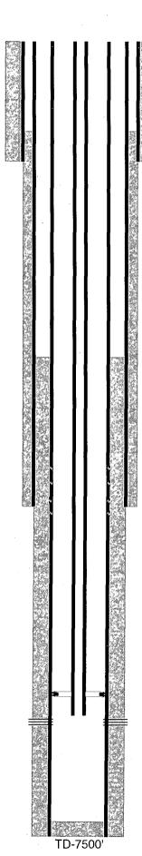
17-1/2" hole @ 1195' 8-5/8" csg @ 1195' w/ 780sx-TOC-Surf-Circ
