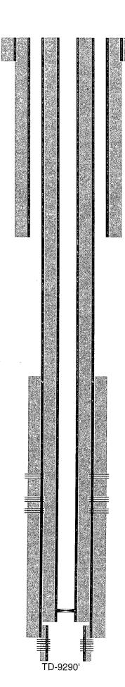
17-1/2" hole @ 331' 13-3/8" csg @ 331' w/ 300sx-TOC-Surf-Circ
