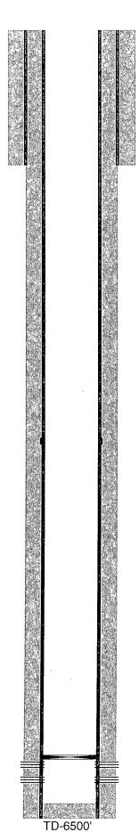
11" hole @ 1100' 8-5/8" csg @ 1100' w/ 500sx-TOC-Surf-Circ
