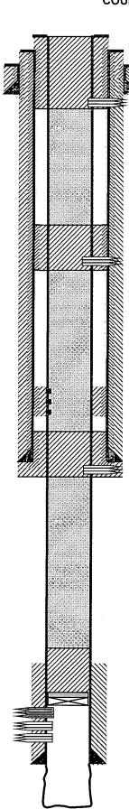
5. PUH & perf @ 211' & sqz 130 sx Class "C" cmt from 211' to surf, CIRC all strings of csg to surf. (Shoe & Water Board)
