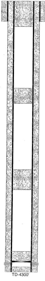
7-7/8" hole @ 4300' 5-1/2" csg @ 4300' w/ 1650sx-TOC-Surf-Circ
