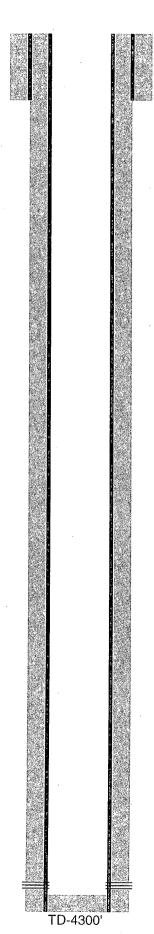
12-1/4" hole @ 356' 8-5/8" csg @ 356' w/ 300sx-TOC-Surf-Circ
