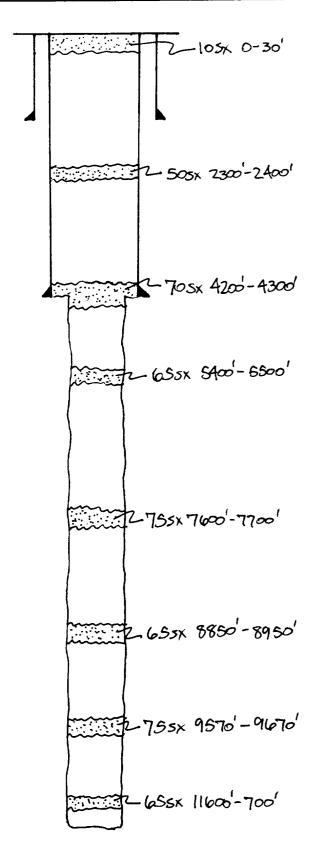
95/8 " casing set at 4250 with 1540 sx of cement.
