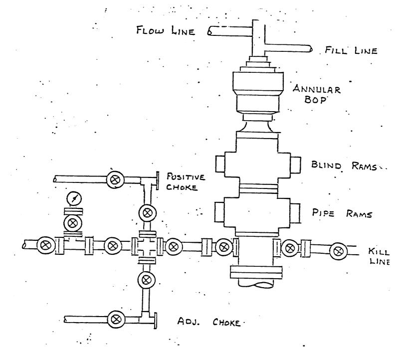
This is to be 3000 psi wp, which is adequate, that will be used on the 11" and 7 7/8" hole. This is the minimum possible BOP stack that will be used. Tenneco may choose to use  $\underline{\text{more}}$  equipment and higher pressure.
