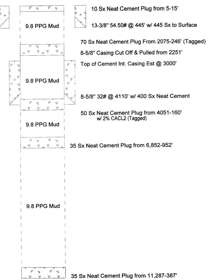
7-7/8" Hole Drilled to 11,387'
