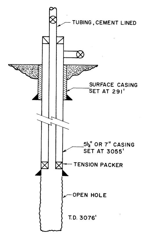
WATER INJECTION WELL SCHEMATIC
