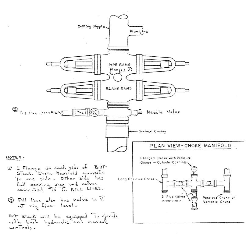
All equipment, piping and valves in BOP arrangement is 900 Series, i.e. 3,000 psi working pressure.
