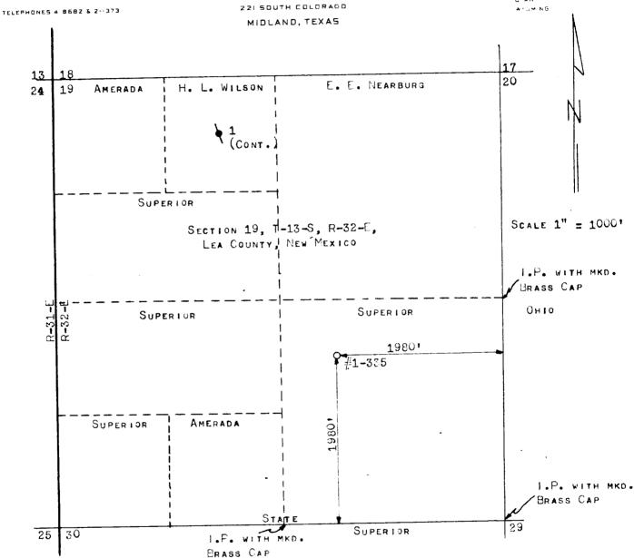
I, W. W. Studdert, Registered Professional Engineer and Land Surveyor. No. 388, State of New Mexico, Hereby Certify that this well location: Superior Oil Co. - State #1-335, 1980' from the South and East Lines of sec. 19, T-13-S, R-32-E, Lea County, New Mexico, was staked on the ground under my supervision and that this plat is true and correct.
