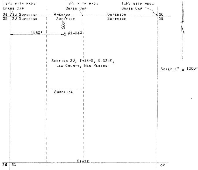
I, W. W. STUDDERT, REGISTERED PROFESSIONAL ENGINEER AND LAND SURVEYOR, No. 388, STATE OF NEW MEXICO, HEREBY CERTIFY THAT THIS WELL LOCATION: SUPERIOR OIL CO. - STATE #1-340, 660' FROM THE NORTH LINE AND 1980' FROM THE WEST LINE OF SEC. 3U, T-13-S, R-32-E, LEA COUNTY, NEW MEXICO, WAS STAKED ON THE GROUND UNDER MY SUPERVISION AND THAT THIS PLAT IS TRUE AND CORRECT.
