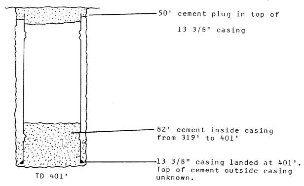
Ran 401' 13 3/8" casing. Mixed 396 sx. cement and pumped in casing. When bottom plug hit shoe and plugged, cement failed to pump out. Pressure went to 1200# and casing parted at top collar in cellar and dropped. Attempted to clean out cement inside casing and found bad casing condition second joint from top and at 338'. Unable to pull casing. 82' cement in bottom of casing 319' to 401'. Placed cement plug in top of casing from surface to 50'. P & A 5-19-58.
