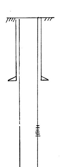
Well capped with 1/4" steel plate
