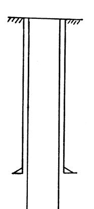
9 5/8" casing set at 340' with 160 Sx of cement Hole size unknown.
