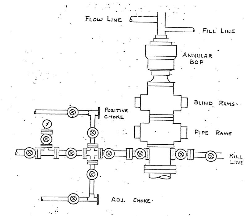
This is to be 3000 psi wp, which is adequate, that will be used on the 11" and 7 7/8" hole. This is the minimum possible BOP stack that will be used. Tenneco may choose to use <u>more</u> equipment and higher pressure.
