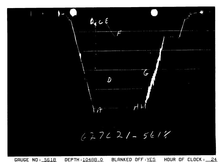
**PRESSURE** TIME ID DESCRIPTION **TYPE** REPORTED CALCULATED REPORTED CALCULATED 5049 5069.1 А INITIAL HYDROSTATIC INITIAL FIRST FLOW 382.7 348 В 13.6 F 15.0 522 502.4  $\mathbb{C}$ FINAL FIRST FLOW INITIAL FIRST CLOSED-IN 522 502.4 С С 62.0 62.9 3256.6 D FINAL FIRST CLOSED-IN 3218 INITIAL SECOND FLOW 609 620.9 Ε F 60.0 59.6 F FINAL SECOND FLOW 1213 1204.6 1204.6 F INITIAL SECOND CLOSED-IN 1213 181.0 182.0 С G FINAL SECOND CLOSED-IN 3218 3215.7 FINAL HYDROSTATIC 5049 4968.3
