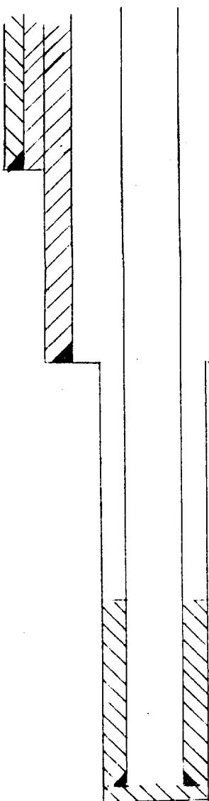
Tabular DataSurface Casing Set at 369'Size 13 3/8 " Cemented with 350 sx.TOC Surface feet determined by CirculationHole size 17 1/2"Intermediate Casing Set at 3293'Size 8 5/8 " Cemented with 1400 sx.TOC Surface feet determined by CirculationHole size 11"Long string Set at 7880Size 4 1/2 " Cemented with 400 sx.TOC 6816 feet determined by temperuture surveyHole size 7 7/8"Total depth 7890Injection interval7577 feet to 7795 feet
