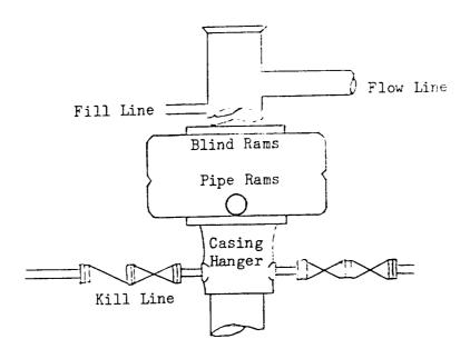
BOP STACK *3000* <del>2000</del> psi working pressure
