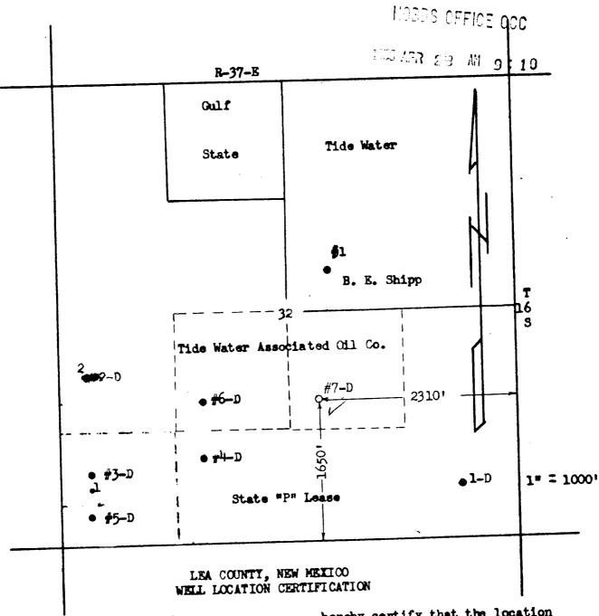
I, J. M. Amis hereby certify that the location for Tide Water Associated Oil Company's Well No. 7-D. State "P" Lease, is located by survey on the ground as represented by this plat.
