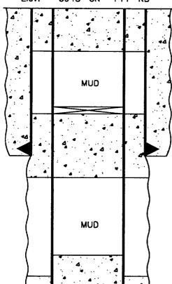
PERFORATE THE 4 1/2" CASING AT 300' CIRCULATE 80 SXS CEMENT THRU PERFS AT 300'
