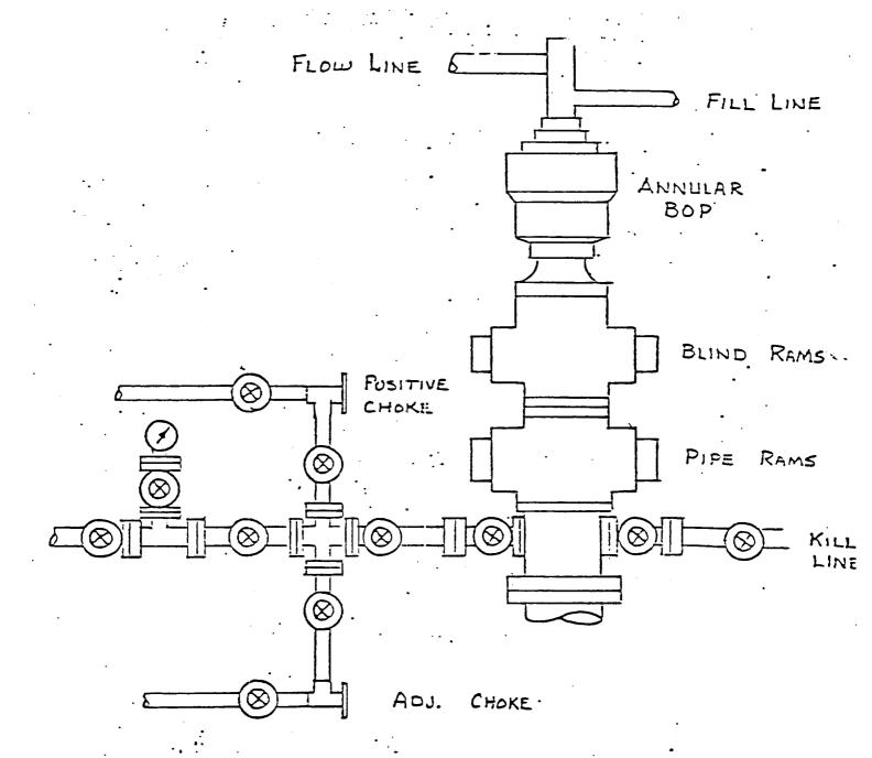
This is to be 3000 psi wp, which is adequate, that will be used on the 11" and 7 7/8" hole. This is the minimum possible BOP stack that will be used. Tenneco may choose to use more equipment and higher pressure.
