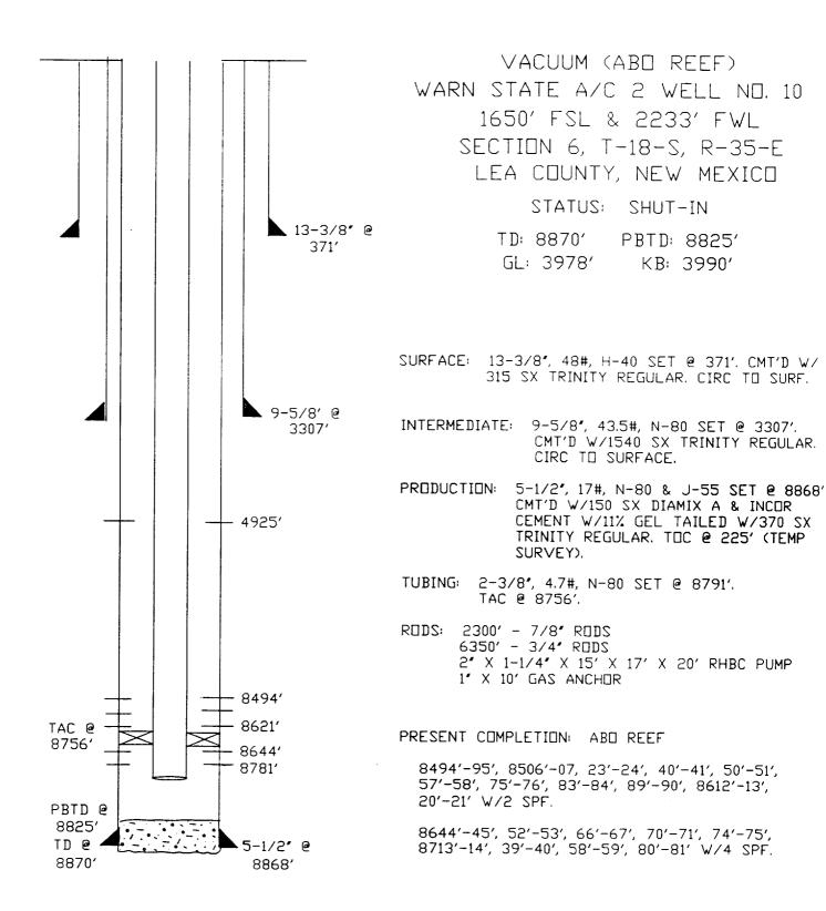
HISTORY: DRILLED IN MAY, 1963. COMPLETED IN ABO REEF F/8494'-8781'. A/2000 GALS. AF/15000 GALS THIN RETARDED ACID. TRIED TO ISOLATE SAN ANDRES/GLORIETTA IN MARCH, 1979 BECAUSE TOC WAS THOUGHT TO BE @ 6155'. PERFORATED CASING W/3 SHOTS @ 4925'. TRIED TO PUMP DOWN TUBING @ 2000#. COULD NOT. TOC WAS LATER DETERMINED TO BE 225' FROM TEMPERATURE SURVEY. SHUT-IN DECEMBER, 1989 AFTER PRODUCING 234 MBD, 771 MMCF, & 18 MBW FROM ABO REEF.
