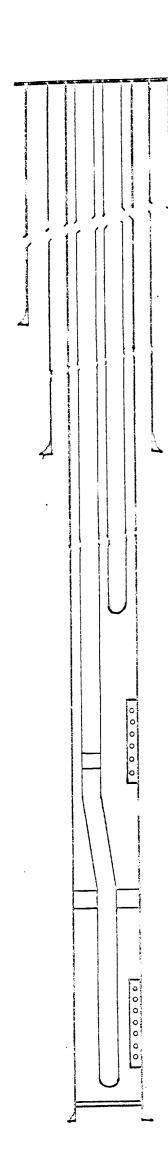
13-3/8" Casing set at 354' with 350 sxs. Cement Circulated.
