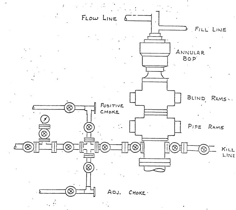
This is to be 3000 psi wp, which is adequate, that will be used on the 11" and 7.7/8" hole. This is the minimum possible BOP stack that will be used. Tenneco may choose to use more equipment and higher pressure.
