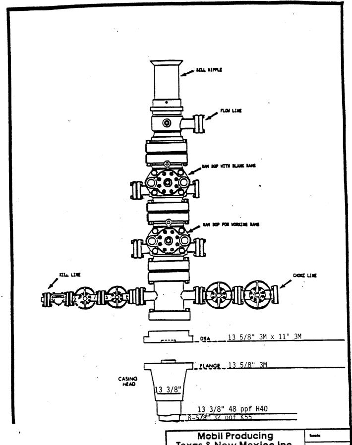
\*NOTE: ALL VALVES ARE METAL-TO-METAL SEAL AND FLANGED.
