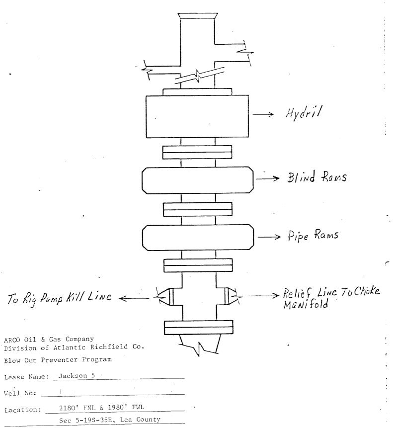
BOP to be tested when installed on well and will be maintained in good working condition during drilling. All wellhead fittings to be of sufficient pressure to operate in a safe manner.
