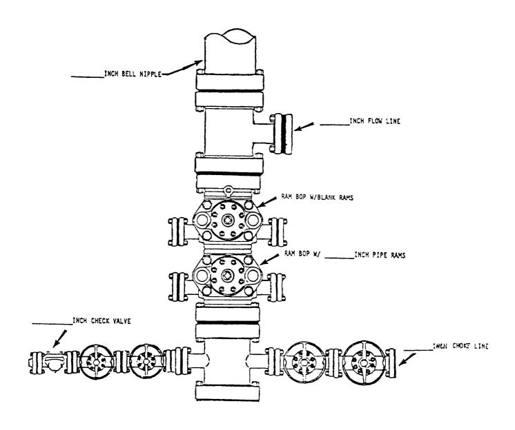
\*HOTE: ALL VALYES ARE METAL-TO-METAL SEAL AND FLANGED, ALL COMPONENTS MUST MEET ABOVE MINIMUM PRESSURE RATINGS. ALL COMPONENTS TO BE TESTED TO RATED PRESSURE AFTER ASSEMBLY AND BEFORE FURTHER DOWNHOLE OPERATIONS MAY BE CONDUCTED.
