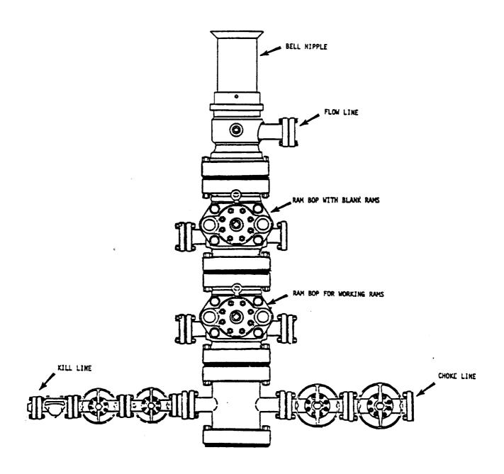
\*NOTE: ALL VALVES ARE METAL-TO-METAL SEAL AND FLANGED.
