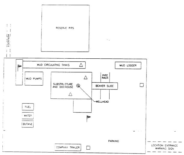
H2S MONITORS WITH ALARMS AT THE BELL NIPPLE, SUBSTRUCTURE, AND SHALE SHAKER WIND DIRECTION INDICATORS
