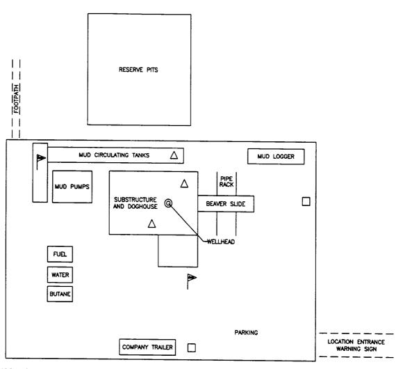
↑ H2S MONITORS WITH ALARMS AT THE BELL NIPPLE, SUBSTRUCTURE, AND SHALE SHAKER WIND DIRECTION INDICATORS
