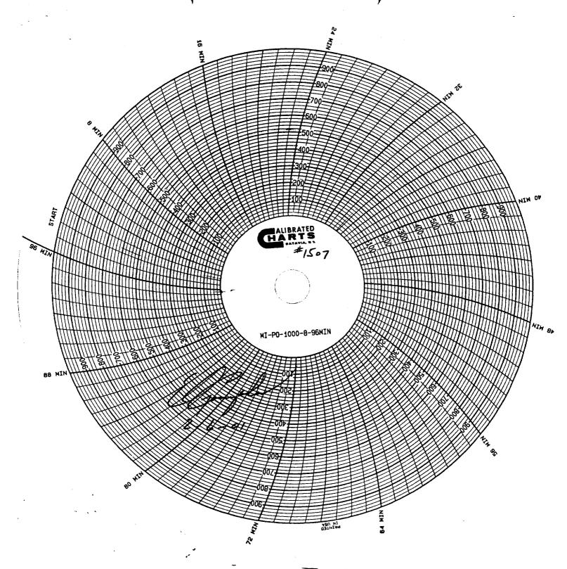
Tested to 540 psi Lost 30 psi in 32 min.
