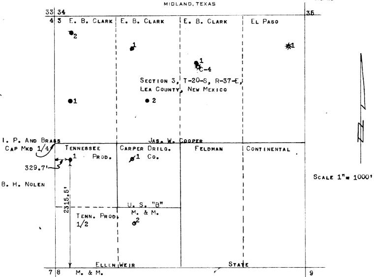
I, Earl K. Monteith, Registered Land Surveyor No. 1317, State of New Mexico, Hereby Certify that this well: Tennessee Production Co.-Ellen Weir #1, 2315.5' from the South Line and 329.7' from the West Line, Section 3, T-20-S, R-37-E, Lea County, New Mexico, was surveyed on the ground under my supervision that this plat is true and correct.
