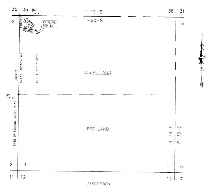
A STRIP OF LAND 50.0 FEET WIDE, 607.9 FEET OR 0.115 MILES IN LENGTH AND BEING 25.0 FEET LEFT AND 25.0 FEET RIGHT OF THE ABOVE CENTERLINE SURVEY.
