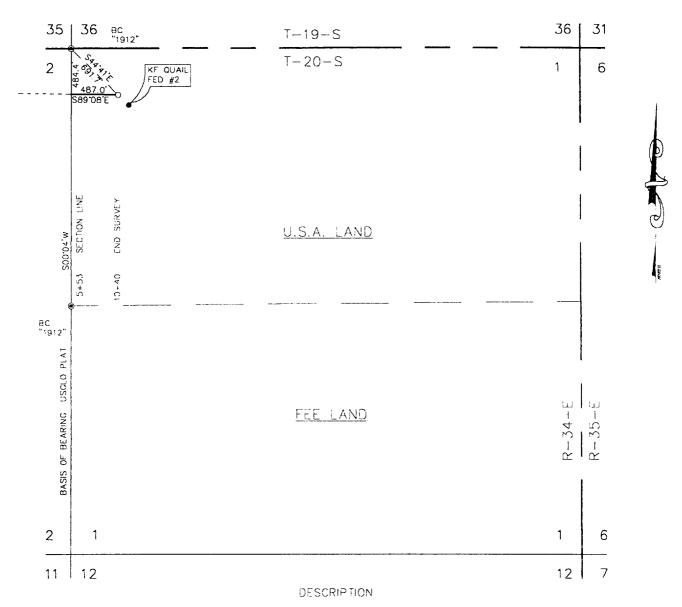
A STRIP OF LAND 50.0 FEET WIDE, 487.0 FEET OR 0.092 MILES IN LENGTH AND BEING 25.0 FEET LEFT AND 25.0 FEET RIGHT OF THE ABOVE CENTERLINE SURVEY.
