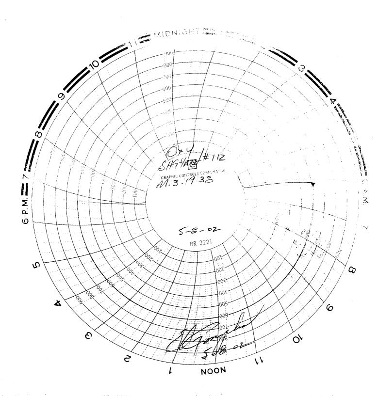
0×9 SHG5/AU+# 112 M.3.19.38 Start PSI 610# Fin 1 605# Tune 31 min Calfdale 5-2-02 Spring 1000# . Clock 60 MIN T/A Stat Tog AST Q Cog 95 -> 2 (3 sec) SURF Q E/Gongalus 5-8-02
