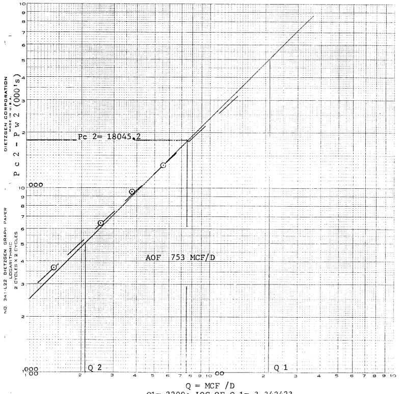
Q = MCF /D Q1= 2200; LOG OF Q 1= 3.342423Q2= 220; LOG OF Q 2= 2.342423N = 1.000
