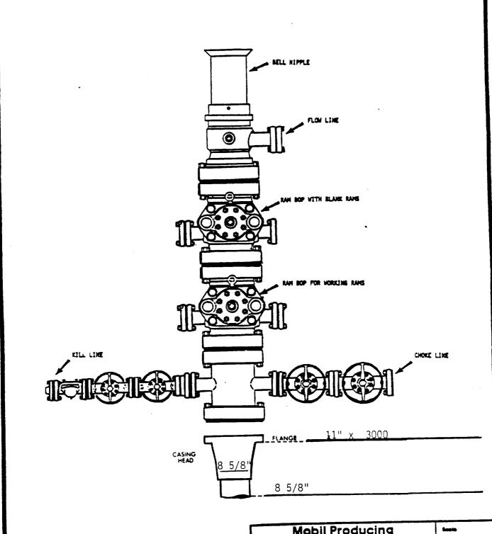
\*NOTE: ALL VALVES ARE METAL-TO-METAL SEAL AND FLAMGED.
