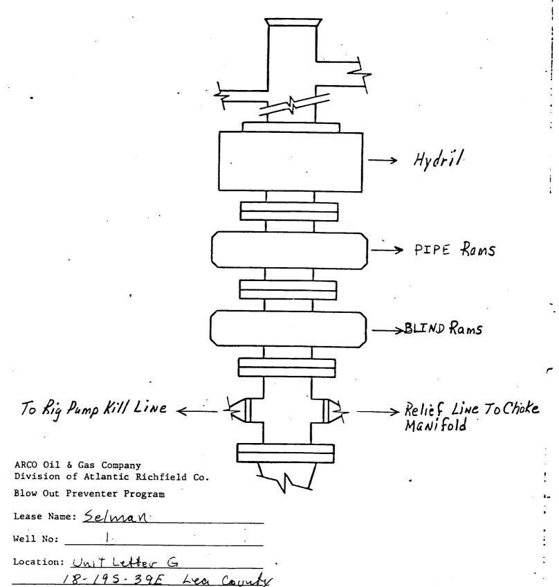
BOP to be tested when installed on well and will be maintained in good working condition during drilling. All wellhead fittings to be of sufficient pressure to operate in a safe manner.
