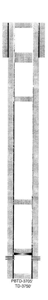
12-1/4" hole @ 438' 8-5/8" csg @ 3750' w/ 260sx-TOC-SURF-CIRC
